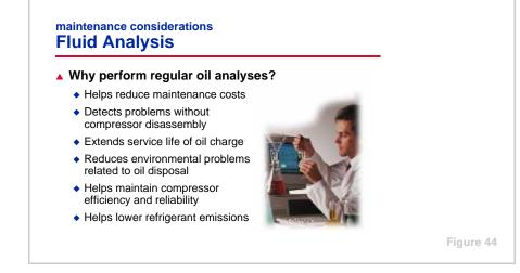
An oil analysis is a key preventive maintenance measure and should be conducted at least annually. It will help the compressor last longer while improving chiller efficiency and reducing refrigerant emissions. A certified chemical laboratory has years of experience in analyzing oil and refrigerant from all types of compressors.
